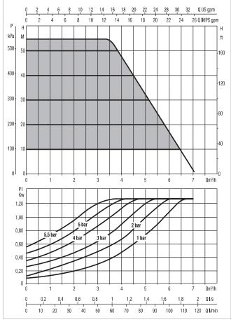
The performance curves are based on kinematic viscosity values =  $1~\text{mm}^2/\text{s}$  and density equivalent to 1000 kg/m³. Curve tolerance according to ISO 9906.
